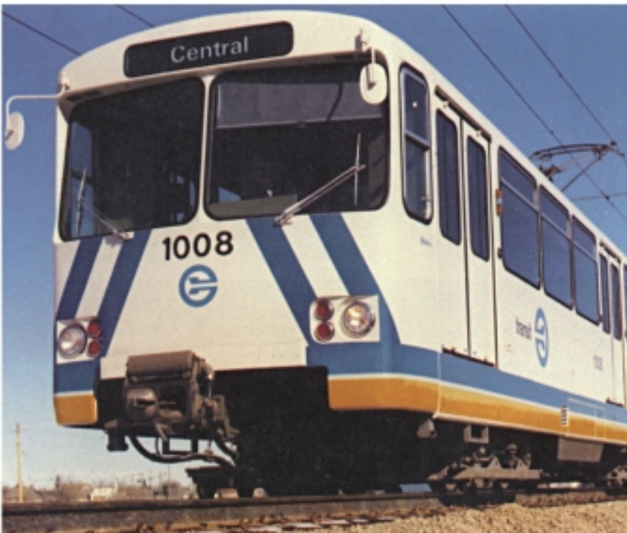
Six-axle articulated rail car of the suburban rail traffic system in Edmonton, Canada ◀
