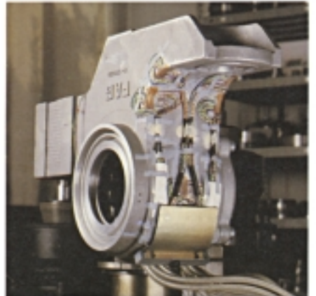
Measuring of stressing by means of strain gauges
